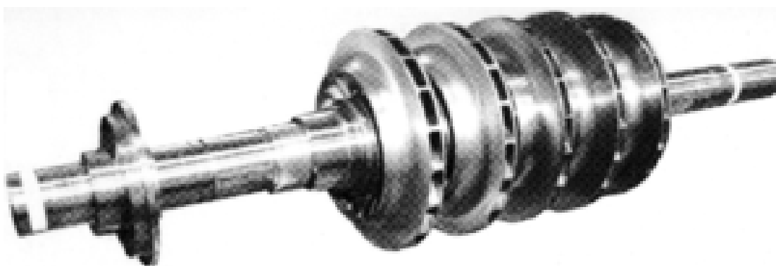
Figure 3.18.2 showing the rotor assembly of a compressor.
