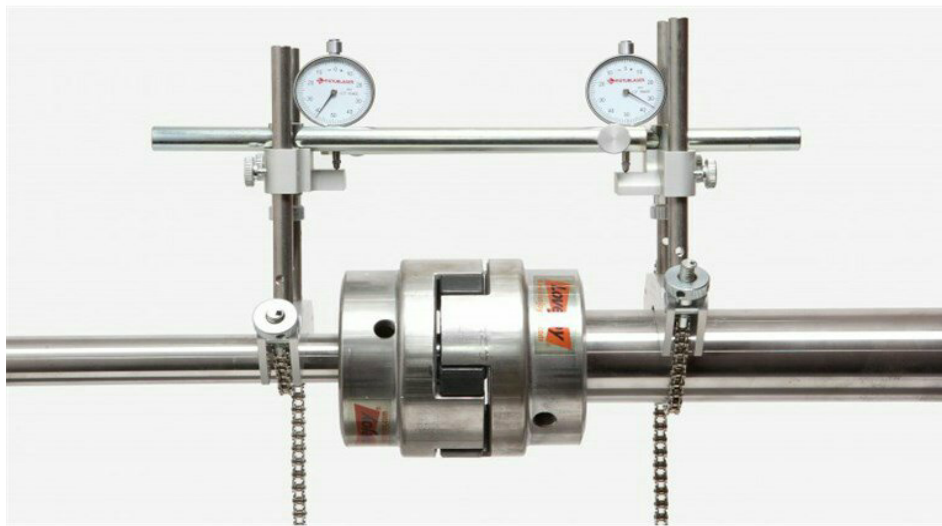
Figure 3.8.1 A diagram depicting the position of the dial indicators on the shafts.
