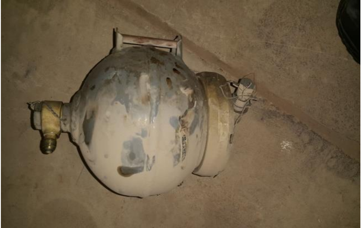
Figure 13 Faulty Hydraulic Accumulator
